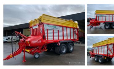
710 O/S Wheels 2M Pickup 35 Double Sided Knives (34mm Theoretical Chop Length) Anti Dirt Roller Fitted LED Lights Full Extra Light Kit Steering Axle Ropes Fitted (Can be Removed) Drive Power from 130hp - Perfect farmers machine Genuine Pottinger Spare Parts Available HP: -
