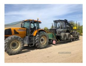
Versatile and durable, Chieftain's stepdeck forestry trailer can be used to transport various forestry harvester and forwarder machines, and even cars. The flat deck and lowered deck make it the ideal choice for various differing machine types and heights
