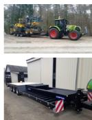
Versatile and durable, Chieftain's stepdeck forestry trailer can be used to transport various forestry harvester and forwarder machines, and even cars. The flat deck and lowered deck make it the ideal choice for various differing machine types and heights
