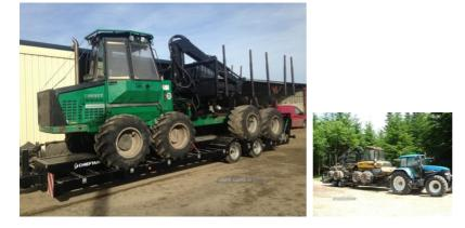
With its heavy duty wheel arches, low bed height and front and rear loading ramps, the Chieftain forestry trailer is specifically designed for the safe and efficient transportation of large forestry harvester and forwarder machines
