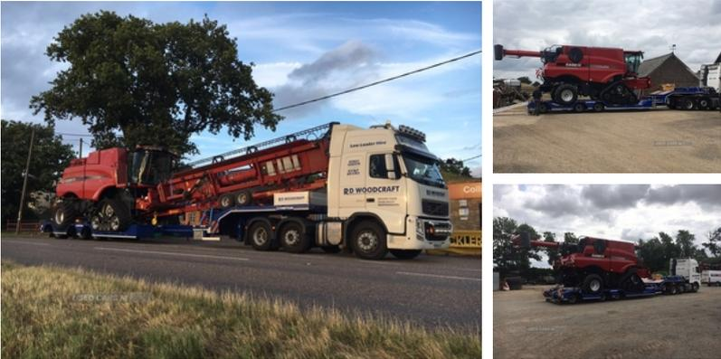
The Combine Trailer specification includes wheel wells on the deck to accommodate the combine's large tyres. The trailer widens from 2.5 metres to 3.5 metres to carry the main body of the combine and extends from 13.6 metres to 18.6 metres.
