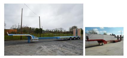
The Chieftain 3 Axle Extendable Semi Low Loader is a strong and robust trailer that is used for the transportation of abnormal loads such as oversized mining equipment, large construction, and agricultural equipment, etc. Various options are available on these models. The trailer comes well equipped with 12.5 Ton full commercial axles (which permit the trailer to travel up to speeds of 105km/h)
