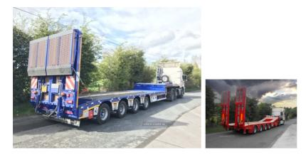
The Chieftain 4 Axle Semi Low-Loader is a strong and robust trailer that is used for the transportation of heavy plant and machinery. The trailer comes well equipped with full commercial axles and air suspension c/w raise and lower valve. (which permit the trailer to travel up to speeds of 105km/h). Standard features also include 2 Rear steering axles
