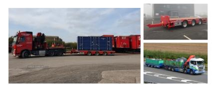
The Chieftain Commercial Flatbed Trailer is a very strong and versatile trailer. With gross weights up to 25 Ton it can also be fitted with ISO Twistlocks to fit a container onto the deck
