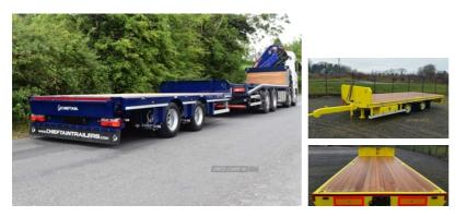
The Chieftain Container trailer has a gross weight up to 11.7 Ton Gross. Fitted with 4 x ISO Twistlocks as standard to fit a  $20^\circ$  Container. The trailer can also be fitted with a removable headboard
