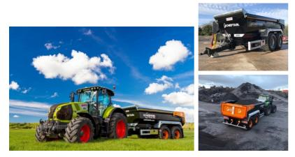
The Chieftain HP20 Fast Tow Dump Trailer is manufactured with Hardox 450 steel as standard. Hardox 450 provides better dent and abrasion resistance as well as longer wear life, so you can achieve even greater savings. This trailer has a lot of unique features including galvanised mudguards and headboard and along with its hydraulic up and over door it is the number one choice for all farmers and contractors.
