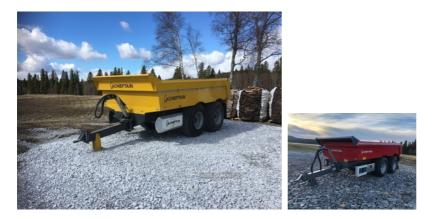
The Chieftain SB12 Dump Trailer is designed for the transportation of materials behind agricultural tractors for up to 40km/h. The SB range includes the option of an invisible door which can be used in conjunction with aluminum ramps to enable the transportation of small machinery. This can be extremely beneficial for customers requiring a multi purpose trailer
