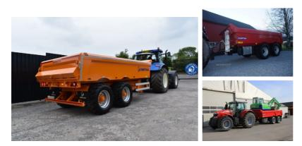
The Chieftain SB16 Dump Trailer is designed for the transportation of materials behind agricultural tractors for up to 40km/h. By choosing the option of an invisible rear door the trailer becomes multi purpose for the loading and transportation of small machinery
