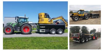
The Chieftain SB16 Fast Tow Dump Trailer is designed for the transportation of materials behind high speed Tractors and Fastracs for up to 60km/h. By choosing the option of an invisible rear door the trailer becomes multi purpose for the loading and transportation of small machinery
