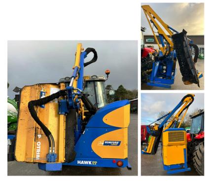
Bomford Hawk5.4 metre reach,LPH joystick controls,Parallel linkage,Oil cooler,Machine running smooth.\*\*Contact Eddie on 07375-104 874 or from ROI 0044 7375-104 874\*\*\*
