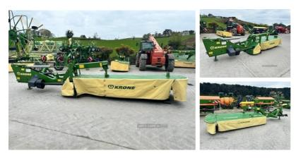
2019 Krone ECR320 10ft  $6^{\prime\prime}$  Disc mower – No condtioner. Safe cut bed c/w quick change blades
